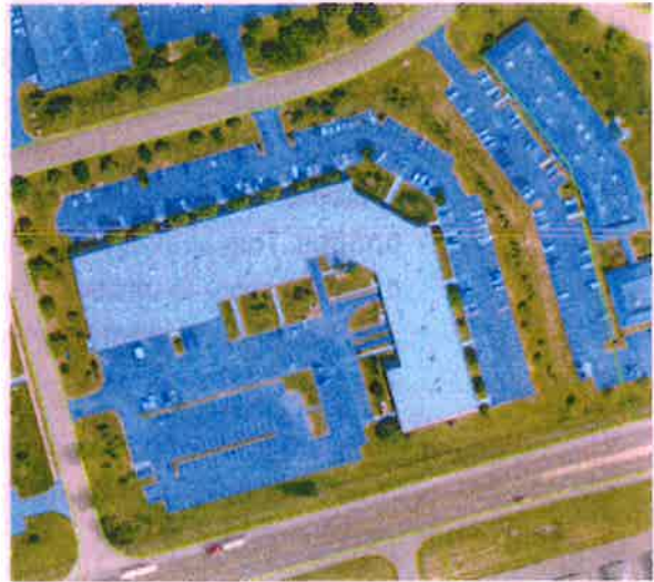
Example of digitized impervious area for a non-single family residential property. Measured impervious area is shown in translucent blue.
