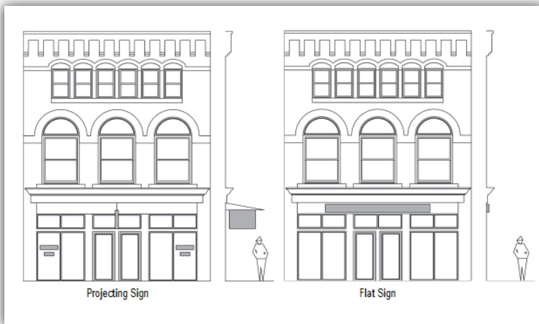
Figure 11: Example of Projecting and Sign Band(Flat) Signs
