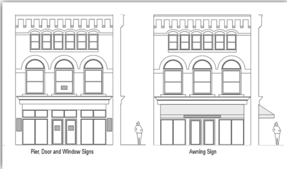
Figure 10: Example of Placement of Pier, Door and Window and Awning Signs
